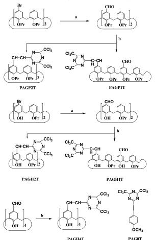
Scheme 1 Preparation of PAGH2T, PAGH1T, PAGP2T, PAGP1T and PAGH4T, Reagents and conditions: a. n-BuLi, THF, -78 $^{\circ}$ C / DMF / H<sub>2</sub>O. b. 2-methyl-4,6-bis(trichloromethyl)-s-triazine, pyridine, acetic acid
